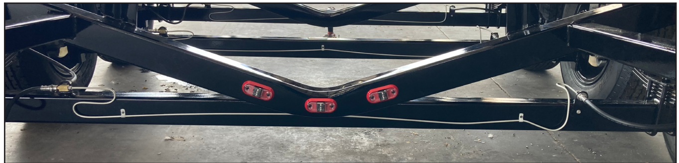
Updated trailer brake line configuration.
